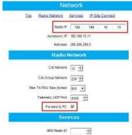
Figure 75 Radio IP Control station
